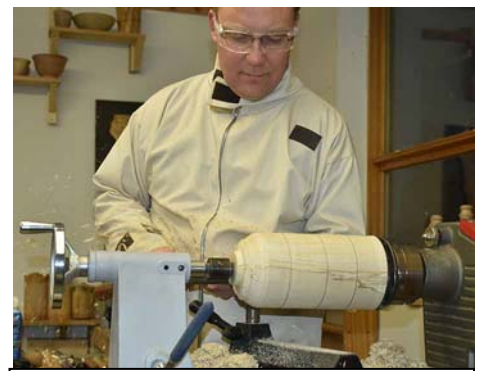
4. Start turning the exterior.
