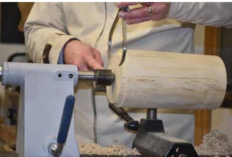
2. Form a tenon to be gripped by your 4-jaw chuck.
