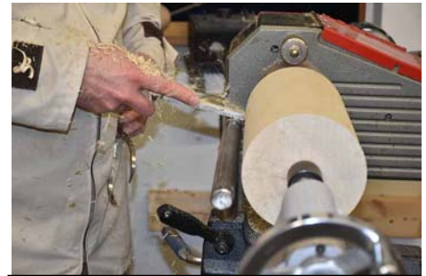
1. Start by forming a cylinder. The workpiece should be at least 1.5 times the length of the final piece.
