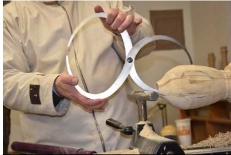
18. Checking the wall thickness with double-ended calipers. Could be thinner but be cautious.
