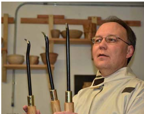
20. Several hollowing tools are needed. A straight tool does the bottom; Curved tools expand the width of the cavity.
