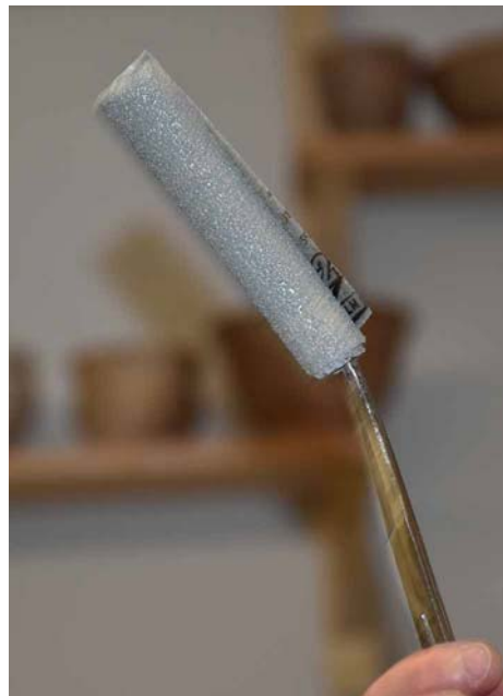
21. Sandpaper wrapped onto forceps help clean up the interior as deep as you can touch.
