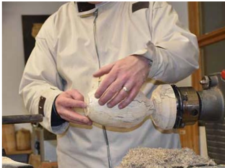
23. Mike is reversing the item after sizing what's left of the base to make a jam-chuck. He'll finish the outside base on the jam chuck.
