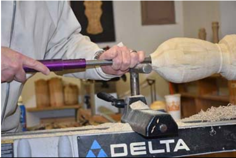
17. Mike has changed tools and is using a side cutter to increase the width of the cavity.
