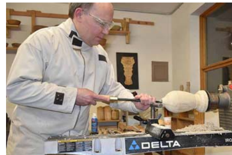
11. Keep a firm grip. Mike uses his body to help control the tool.
