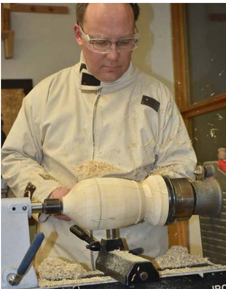
5. The item is taking shape. Note that the tail stock is still in use.
