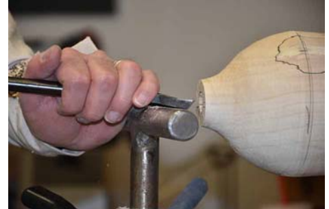
9. Starting at the neck and enlarging the entrance hole.
