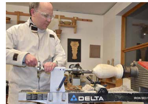
6. Mike is boring out a center hole with a twist-bit. He'll go down most of the way to the interior bottom he has planned.
