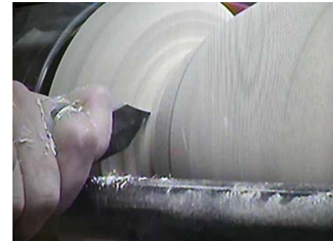
22. Starting to part off the base.
