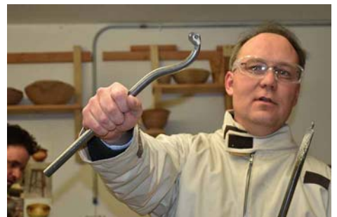
16. This is a hooked interior scraper.
